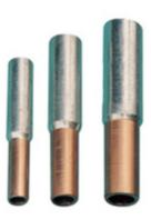
GL aluminiu connection tube is used for the linking of copper core cable,GT series lil-blocking type connection pipe is machined with T2 bar copper,GT series through-hole type connection pipe is pressed with T2 copper pipe
